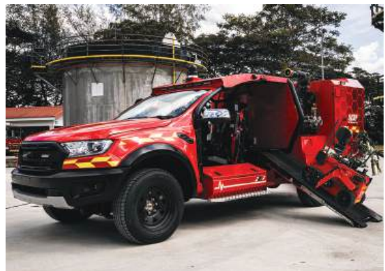
SCDF's 6th Generation Light Fire Attack Vehicle with the Red Rhino Robot (3R) which is able to detect and move towards heat sources autonomously, and spray water and compressed air foam on fires
